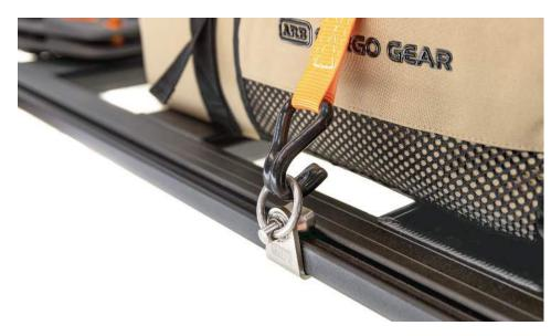
Quick-attach spring-loaded tie-downs are easy to use with a simple one-handed operation. Great for one-off needs and quick loading and unloading.
