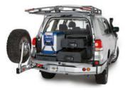
Modular in design for user customisation, Outback Solutions drawers can maximise the versatility of your vehicle's cargo space by being configured with fridge roller drawers, roller floors or stackable drawers. Manufactured from galvanised stainless steel with sealed roller bearings and commercial grade carpet for durability.
