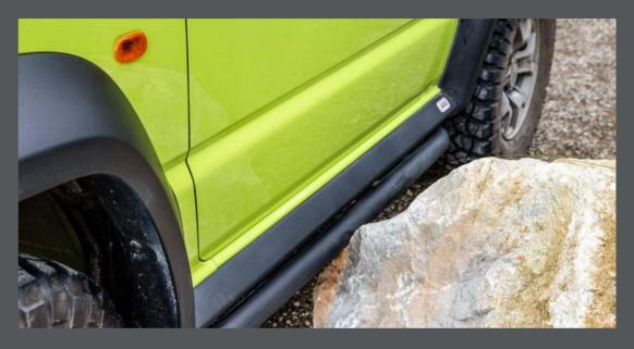
ARB Rock Sliders have been specifically designed for the MY19 Jimny and are located in parallel to the vehicle to provide protection to its vulnerable sills.
